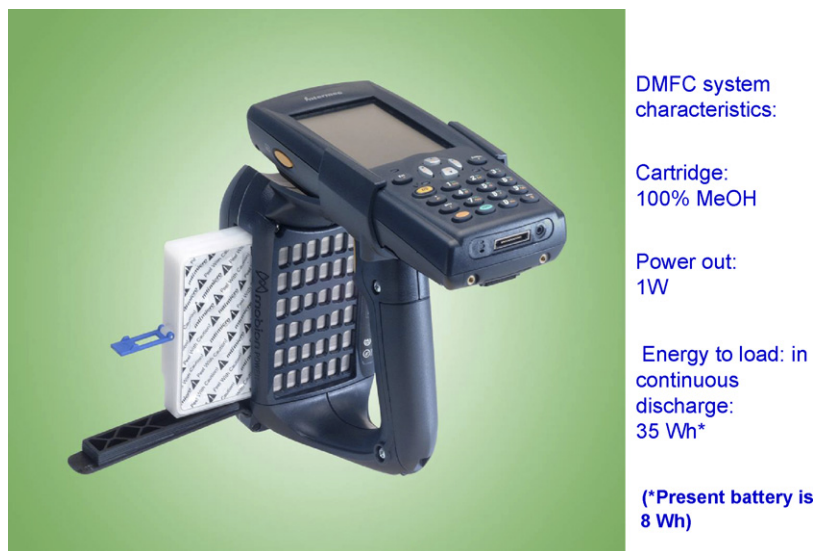
Fig. 9. Air breathing DMFC power system including a flat cell array and methanol cartridge with 100% methanol (directly fed to the anode), integrated into the handle of a RFID tag reader.
